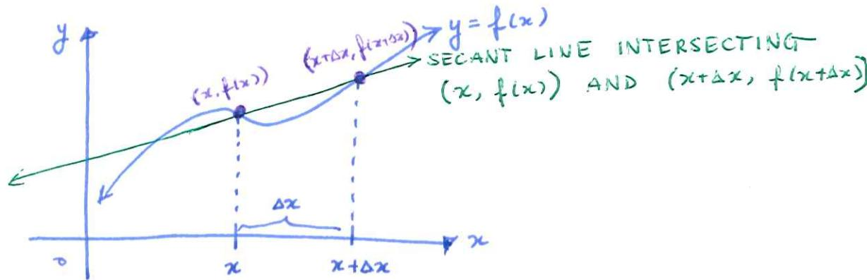
SLOPE OF SECANT LINE ABOVE :  $m_s = \frac{\text{rise}}{\text{run}} = \frac{\Delta y}{\Delta x} = \frac{f(x + \Delta x) - f(x)}{(x + \Delta x) - x}$
