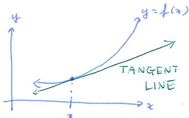
A line tangent to ~~the~~ the graph of  $y = f(x)$  at the point  $x$  intersects the graph locally only at the point  $(x, f(x))$ .
